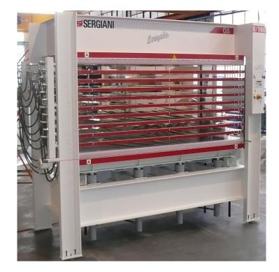
PRESSES GSA FOR DOOR FINISHING . MANUAL COMPOSITION, AUTOMATIC LOADING and MANUAL UNLOADING. "STAND ALONE" PRESSES NOT INSERTED IN LINE.
