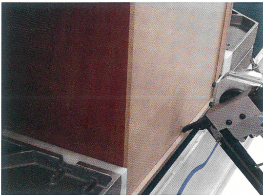
Nailing robot during the cramping of the rear panels Nailing programs with WoodWOP-programming
