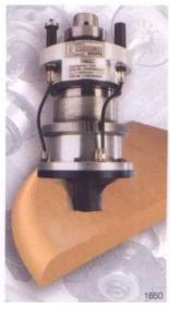
Routing vertical with tracing ring
