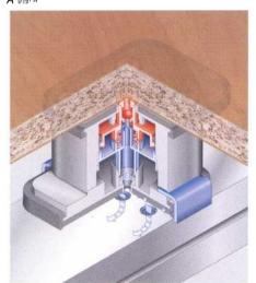
Functioning principle - parallel vacuum system within the pod
