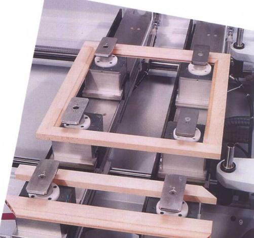
Multi clamping system (i. e. for frame parts)
