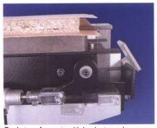
Backstops for parts with laminate and veneer overhang
