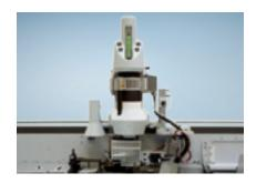
**PU pre-melting unit** Melting output 6 kg/h. With KAL 370 profiLine.
