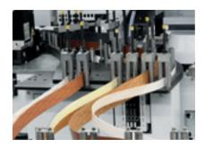
**6-slot magazine**Automatic infeed of six different edges.
