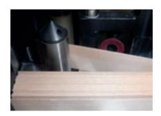
**Suction cup for strip separation**Separation of strips from a package.
