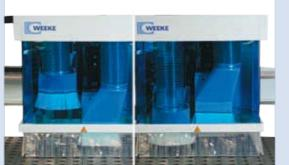
Efficient dust extraction - the dust extraction is separated to each working unit (router or drilling unit)
