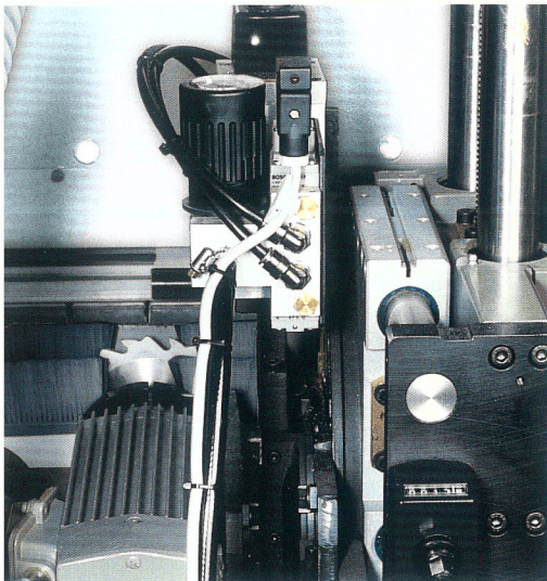
Universal trimming unit UF 11 For grooving, rebating and profiling with swivel-action and controlled motor.
