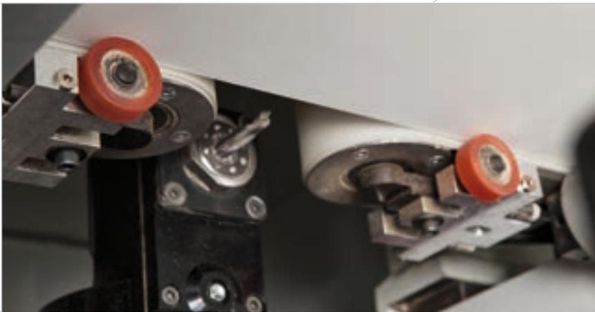
Patented dual-section haul-off for machining the 4 panel edges without limits (not available on Vektor 25 and 30).
