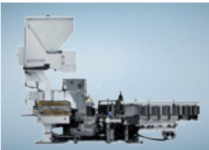
**Hot-melt gluing unit with solid wood package**
