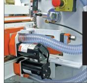
Dual post cleaners with top and bottom rotary brushes, rotate against the workflow to cleanly remove foil feathering to smooth the top and bottom foil trim line from the profiled edges as the part exits the outfeed. An adjustable mini cooler cools the foiled edges prior to entering the post cleaner station.
