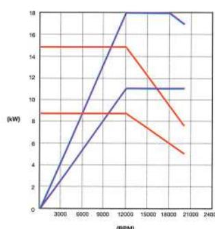
**"High power"** electro spindles Maximum power up to 20,000 rpm for intensive machining with high rates of stock removal.
