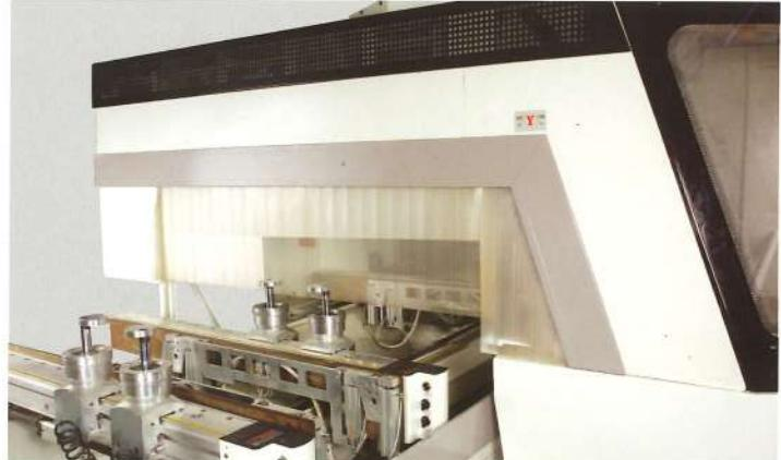
Side protection strips can be excluded by CNC to allow high speed movements.
