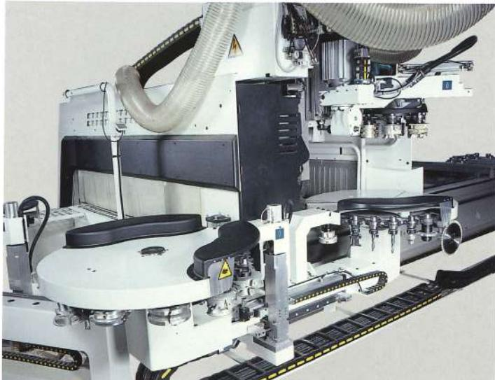
Both machining units can take the required tools from tool magazines positioned on the mobile beam enabling the machine to be ready for any type of application.
