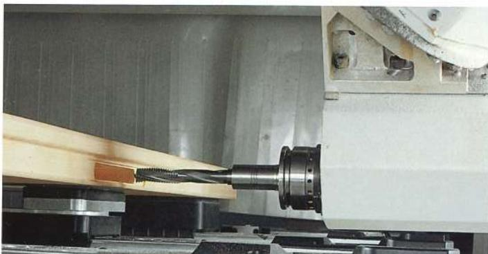
Thanks to the small dimensions of the PRISMA K 5 axis unit, there is no need to raise the component when machining on the horizontal axis because the Z axis stroke is utilised to the maximum. It is also possible to carry out saw cutting on very thick components.
