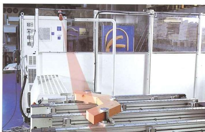
Guided by a laser light, the operator can easily position arched components.
