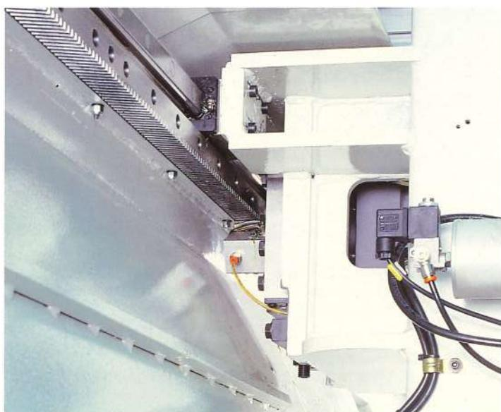
Helical tooth racks for maximum precision on high speed movements.
