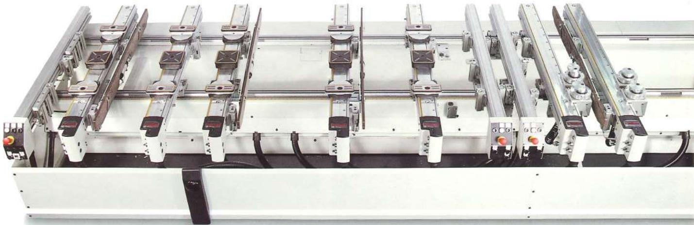
TVN worktable bars are the perfect solution for quick and safe component clamping: the bars can be fitted with quick release suction cups or pneumatic clamps for maximum ease of use.
