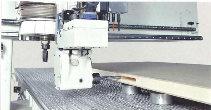
Fixed or CNC controlled **Universal K2** unit for continuous horizontal-axis machining.
