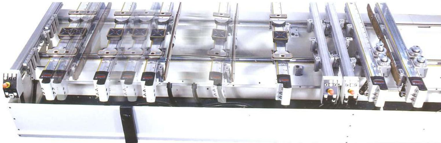
TVN SET is the ideal worktable for the automatic positioning of the bars for linear components such as doors, windows, staircases, beams, columns. Extremely simple and easy to use, this system combines the flexibility of clamping device manual positioning with automatic bar positioning handled by the CNC.
