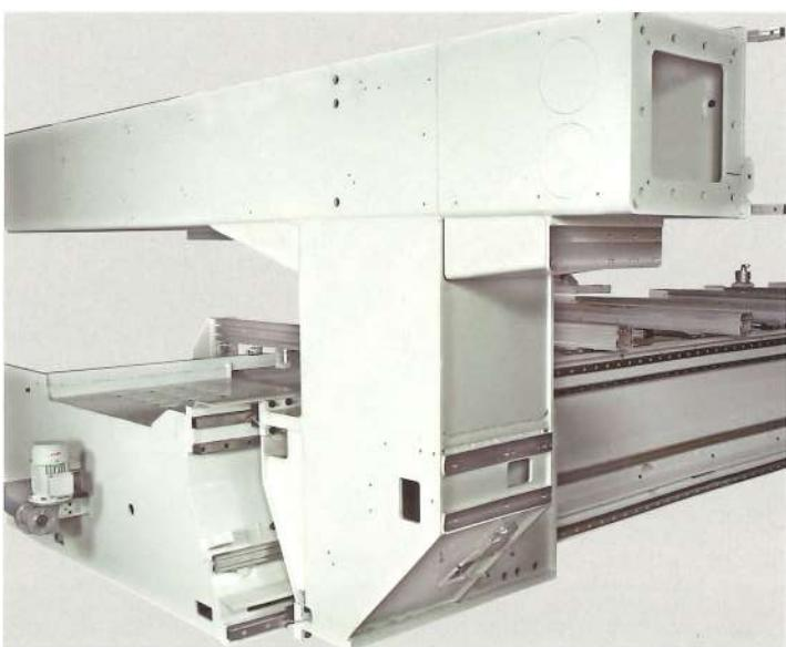
Machine base and mobile beam are manufactured with an electro-welded steel structure and stabilized with thick steel sheets and stiffening ribs. The structure is machined on CNC Machining Centres in one single location in order to guarantee the highest degree of flatness, perpendicular structure and precise tolerances.
