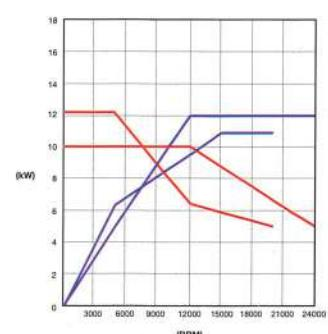
**"High flexibility"** electro spindles The correct balance between power and rotation speed. The multi-purpose electro-spindles are ideal for using a 5 axis machining head.
