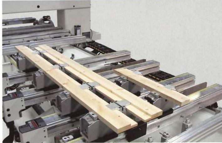
Doorpost machining is precise and safe thanks to special pneumatic clamps.
