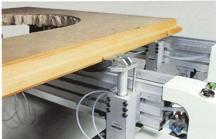
Reference stops ideal for the trimming of veneered panels with overhanging projections.
