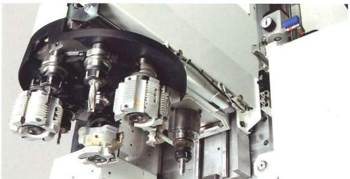
**PBTC:** Auxiliary routing unit with automatic tool changer to ensure the production cycle is faster.
