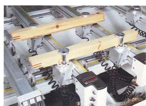
For flexible window production, it is required to have a practical, fast and intuitive system that can quickly fit each window dimension. TVN SET fully meets this requirement: just equip the bars with suction cups or with pneumatic clamps and then modify window dimension data in the parametric program according to size of the window to be machined. The bars automatically position themselves to fit to the new dimensions.
