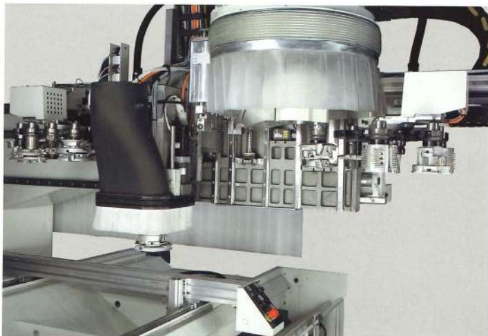
TECNO machining head considerably increases productivity enabling tool changing in masked time during other auxiliary unit machining cycles.
