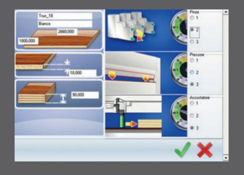
DIFFERENT PRESSURES: THE BEST RESULT FOR ZERO SET-UP TIMES. Very fast work changeover due to the possibility of presetting. The automatic and independent management of the pressure beam, clamps and side alignment device according to the type of material to be cut allows perfect machining both on soft and deformable panels and also on hard ones (opt.).
