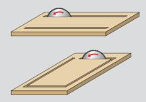
**SLOTS EXECUTION DEVICE: AT THE OPERATOR'S SERVICE.** This particular device allows the carrying out of interrupted cuts inside the panel for producing, for example, slotted doors (opt.).
