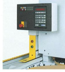
The newly developed modular control system is very user-friendly in addition to offering optimal service ease. Both machines are already fully equipped for remote servicing via modem - the wave of the future. The red/green traffic mode controls show the operator when the next workpiece can be loaded.
