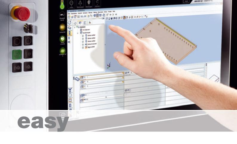
At the focus of this solution is a large multi-touch monitor in widescreen format, which is used to control machine functions by direct touch contact. The entire user interface has been optimized for touch operation and offers an array of help and assistance functions designed to radically simplify the work experience. Standardized control elements and software modules ensure that all HOMAG Group machines can be operated in
