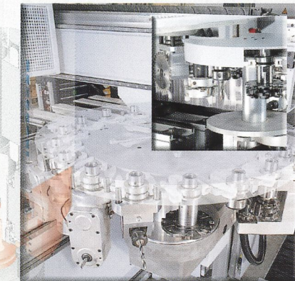
8-fold or 18-fold tool changer in X-direction
