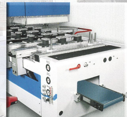
A chip transport belt can be integrated in the rigid machine frame as an option.
